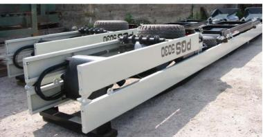
Mobile, radial, troughed belt conveyors, fitted with 3 ply / 30" 750 mm wide conveyor belting with a vulcanised joint (chevron belt available as an option). Feed boot (with extended sides as standard), support pivot and fully guarded
